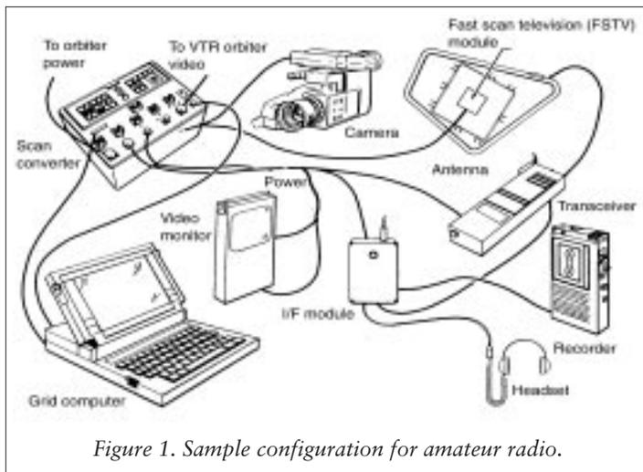
Figure 1. Sample configuration for amateur radio.
